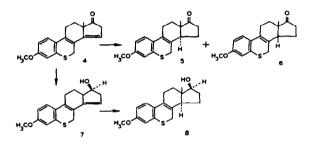
To circumvent the unfavourable <u>cis/trans</u> ratio of the mixture obtained upon hydrogenation, the ketone <u>4</u> was reduced with  $\operatorname{HaBH}_4$ when alcohol <u>7</u> (m.p. 94-101°) was obtained in 70% yield. IR 7  $\operatorname{Max}^{\operatorname{KBr}}$  3450 cm<sup>-1</sup> (OH); UV  $\lambda \operatorname{EtOH}_{\operatorname{Max}}$  225 (14800), 276 (23000) and 323 (13700) nm;
